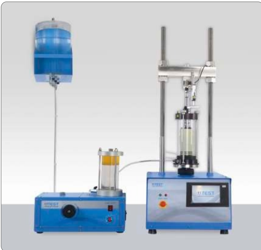
UU Only Triaxial Test Configuration
