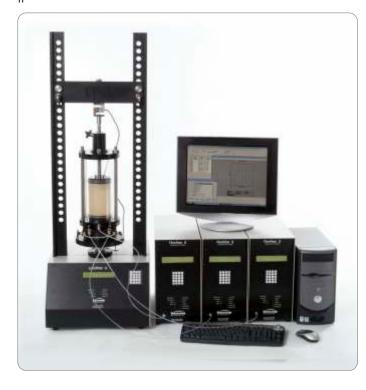
The LoadTrac II/FlowTrac II flow pump provides a unique and versatile way to run flexible wall permeability tests on a wide variety of materials quickly and accurately. By adjusting the gradient or the flow rate across the sample, the system can measure permeabilities of cohesive soils varying from 10-4 cm/sec to 10-9 cm/sec. With the appropriate test cells, this one system can determine the permeability of some silty clays within minutes.
