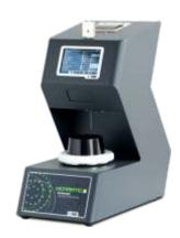
The setting time determination of cement/mortar/gypsum is one of the most important parameter for the quality inspection and verification.
