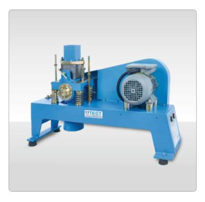
The UTCM-0930 Vibrating Machine is used for the preparation and compaction of 70.7 mm mortar cube specimens.
