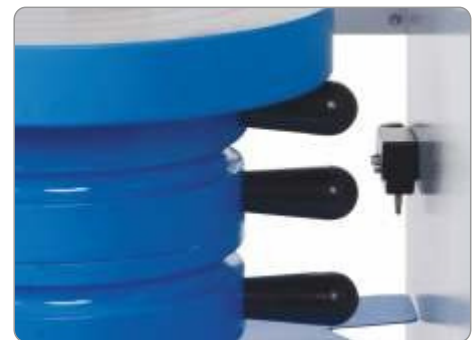
Loading Cylinder Assembly and Limit Switch
