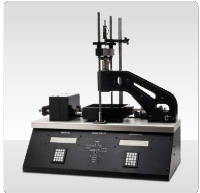
Standard Fully-Automated Rock Shear System
