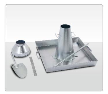
• Slump Cone Top Dia: 100 ±2 mm / Base Dia: 200 ±2 mm/ Height: 300 ±2 mm /Thickness 1,5mm Slump Base Plate 500x500x60 mm with Handle with UTC-0400E) • Slump Base Plate with Handle and Clamps with UTC-0398E) Slump Funnel, Galvanized Steel Tamping Rod Ø 16x600mm Round Scoop, medium Steel Ruler 300x1mm
